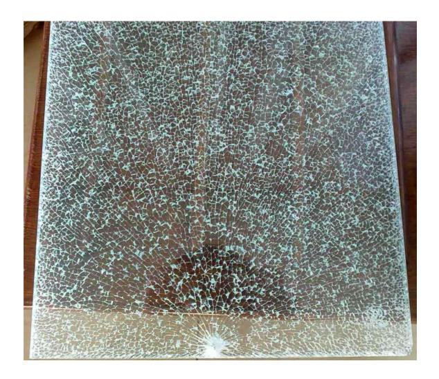
Tempered laminated glass is designed to shatter into small pieces, preventing possible injury. When both pieces of glass are broken it produces a "wet blanket" effect and it will fall out of its opening.
