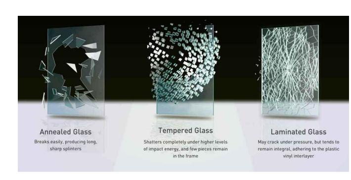
Laminated glass is manufactured by bonding two or more layers of glass together with an interlayer, such as PVB, under heat and pressure, to create a single sheet of glass. When broken, the interlayer keeps the layers of glass bonded and prevents it from breaking apart. The interlayer can also give the glass a higher sound insulation rating.
