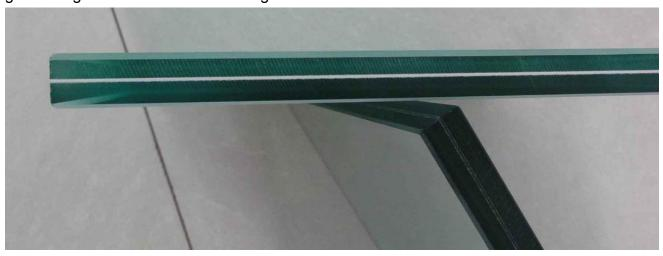
Laminated glass that is made up of annealed glass is normally used when safety is a concern, but tempering is not an option. Windshields are typically laminated glasses. When broken, the PVB layer prevents the glass from breaking apart, creating a "spider web" cracking pattern.
